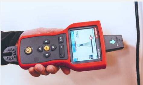
Non-contact voltage (NCV) detection.
